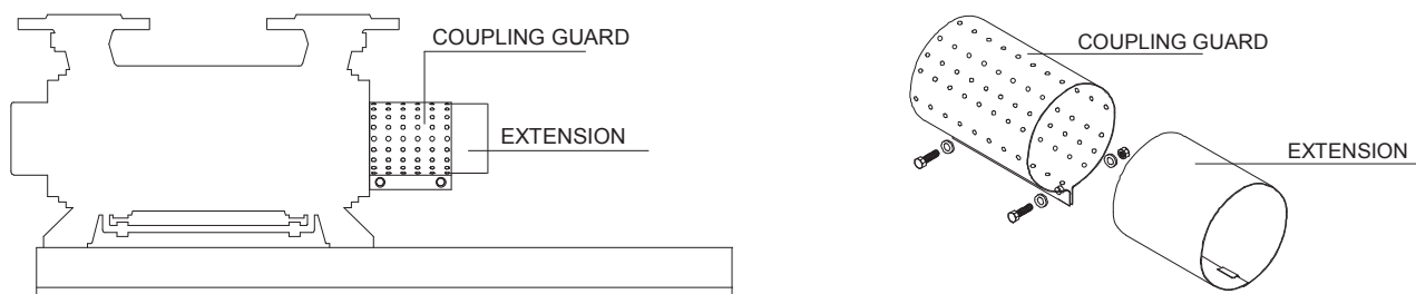
Fig. 18 - MOUNTING THE UNITS ON THE BASEPLATE
